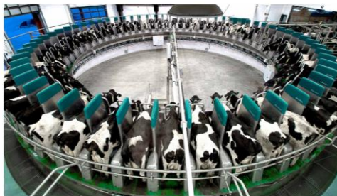
GEA's DairyProQ milking parlor is capable of milking up to 400 cows per hour with one operator.
