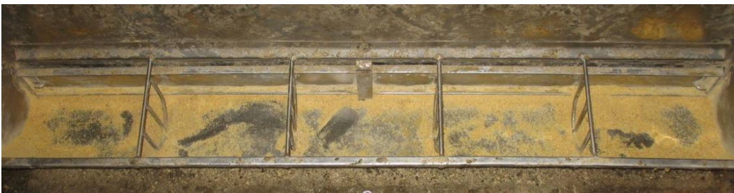
Figure 6. Feeder setting 3, 55% of the pan is covered
