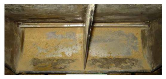
Figure 1. Narrow feeder adjustment (minimum feeder gap was 0.5 in. with a maximum gap of 0.75 in.) averaged 27% feeder pan coverage.
