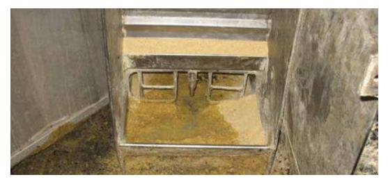
Figure 7. Wet-dry feeder at setting 18 with a 1.25-in. opening and ≈87% pan coverage.
