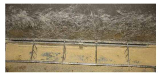
Figure 6. Conventional dry feeder at setting 10 with a 1.09- to 1.35-in. opening and ≈79% pan coverage.
