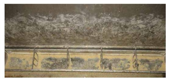
Figure 5. Conventional dry feeder at setting 8 with a 0.80- to 1.07-in. opening and  $\approx$ 21% pan coverage.
