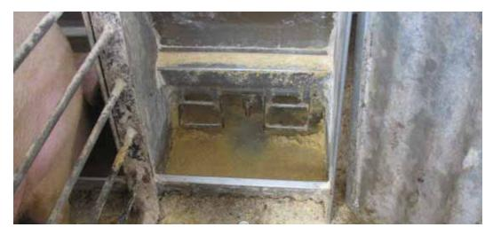
Figure 4. Wet-dry feeder at setting 10 with a 0.75-in. opening and ≈63% pan coverage.
