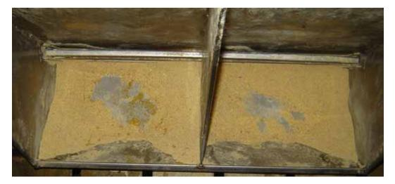
Figure 2. Medium feeder adjustment (minimum feeder gap was 0.75 in. with a maximum gap of 1.00 in.) averaged 58% feeder pan coverage.
