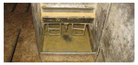
Figure 3. Wet-dry feeder at setting 14 with a 1.00-in. opening and ≈65% pan coverage.
