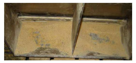
Figure 2. Wide feeder adjustment (minimum feeder-gap opening was 1.00 in. with a maximum gap of 1.25 in.) averaged 83% feeder pan coverage.
