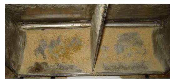
Figure 1. Narrow feeder adjustment (minimum feeder-gap opening was 0.5 in. with a maximum gap of 0.75 in.) averaged 45% feeder pan coverage.
