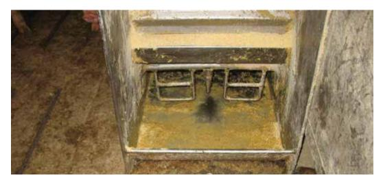
Figure 2. Wet-dry feeder at setting 10 with a 0.75-in. opening and ≈57% pan coverage.
