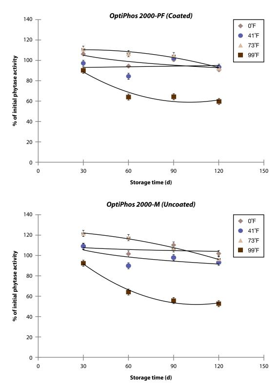
Figure 1. Residual phytase activity (% of initial) for OptiPhos 2000-PF (coated) and Opti-Phos 2000-M (uncoated) as affected by storage temperature (freezer [0°F], refrigerator [41°F], at room temperature [73°F], and in a controlled environment chamber [99°F and 75% humidity]) and time (30 to 120 d). Each data point (least square mean ± 2.32) is the mean of 3 observations.
