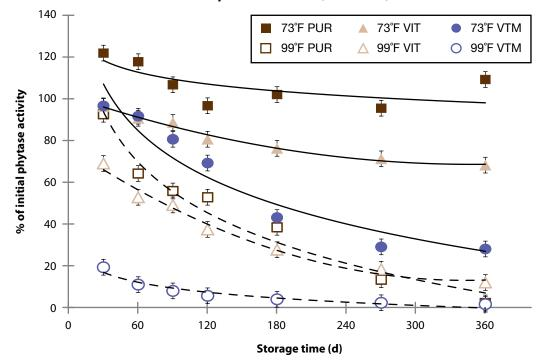
Figure 4. Residual phytase activity (% of initial) for OptiPhos 2000-PF (coated) and OptiPhos 2000-M (uncoated) as affected by form of storage (as pure product [PUR], in a vitamin premix [VIT], or in a vitamin-trace mineral premix [VTM]), storage temperature (room temperature [71°F], and in a controlled environment chamber [99°F and 75% humidity]) and time (30 to 360 d). Each data point (least square mean ± 3.75) is the mean of 3 observations.
