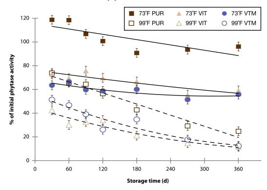
Figure 5. Residual phytase activity (% of initial) for Phyzyme 10000 TPT (coated) and Phyzyme 5000G (uncoated) as affected by form of storage (as pure product [PUR], in a vitamin premix [VIT], or in a vitamin-trace mineral premix [VTM]), storage temperature (room temperature [73°F], and in a controlled environment chamber [99°F and 75% humidity]) and time (30 to 360 d). Each data point (least square mean ± 3.75) is the mean of 3 observations.
