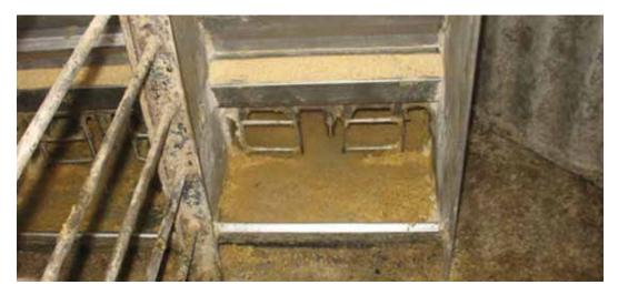
Figure 3. Wet-dry feeder at setting 14 with a 1.00-in. opening and ≈83% pan coverage.
