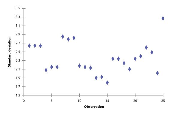
Figure 2: Geometric standard deviations (sgw) from 25 observations of a single sample
